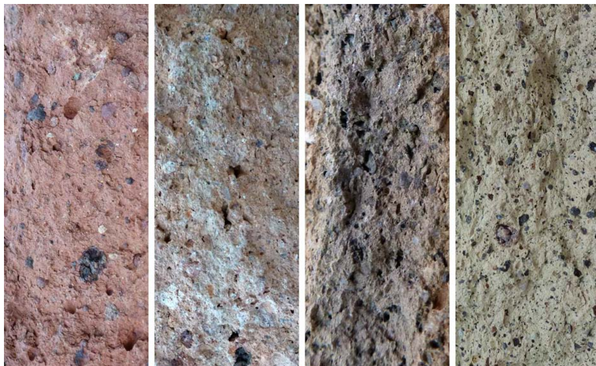
Fig. 1. Macroscopic photographs of cores (fresh breaks) of Groups I through IV fabrics (from left to right) architectural terracottas, Satricum acropolis. Each strip is about a cm (photo M. Gnade).
